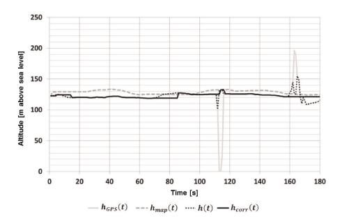
Figure 3 Comparison between the corrected altitude profile  $h_{corr}(t)$  and the smoothed and interpolated altitude  $h_{int,sm,1}$
