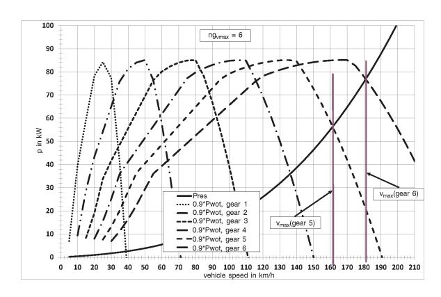
$\label{eq:Figure A2/1b} \textit{An example where } \textbf{ng}_{\text{max}} \; \text{is the } \textbf{2}^{\text{nd}} \; \text{highest gear}$
