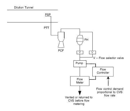
$\label{eq:Figure A5/13}$  Double dilution particulate sampling system
