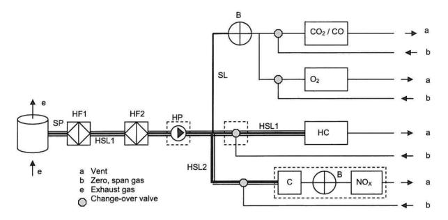
Figure 1 - Arrangement of exhaust gas analysis system
