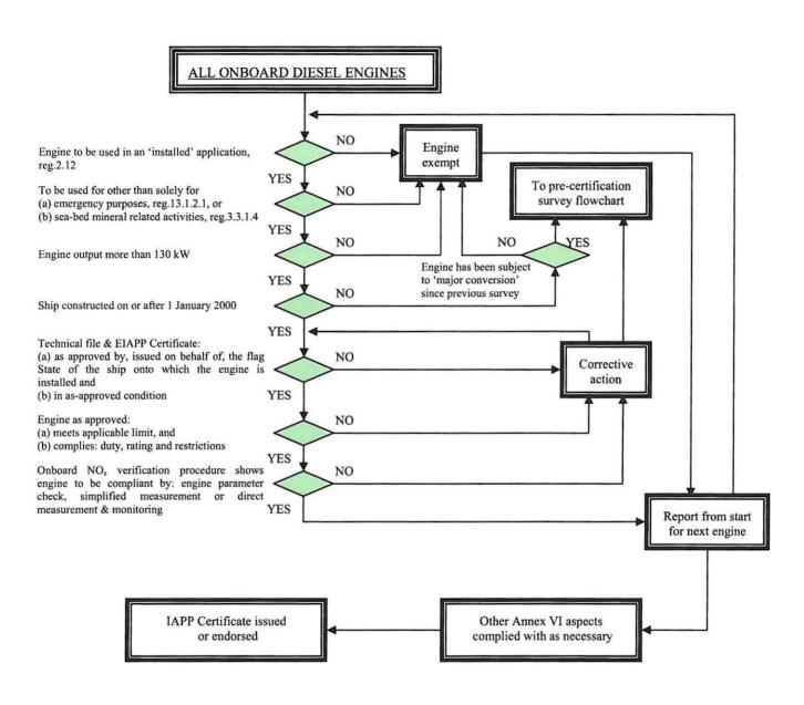
Figure 3 - Renewal, annual or intermediate survey on board a ship
