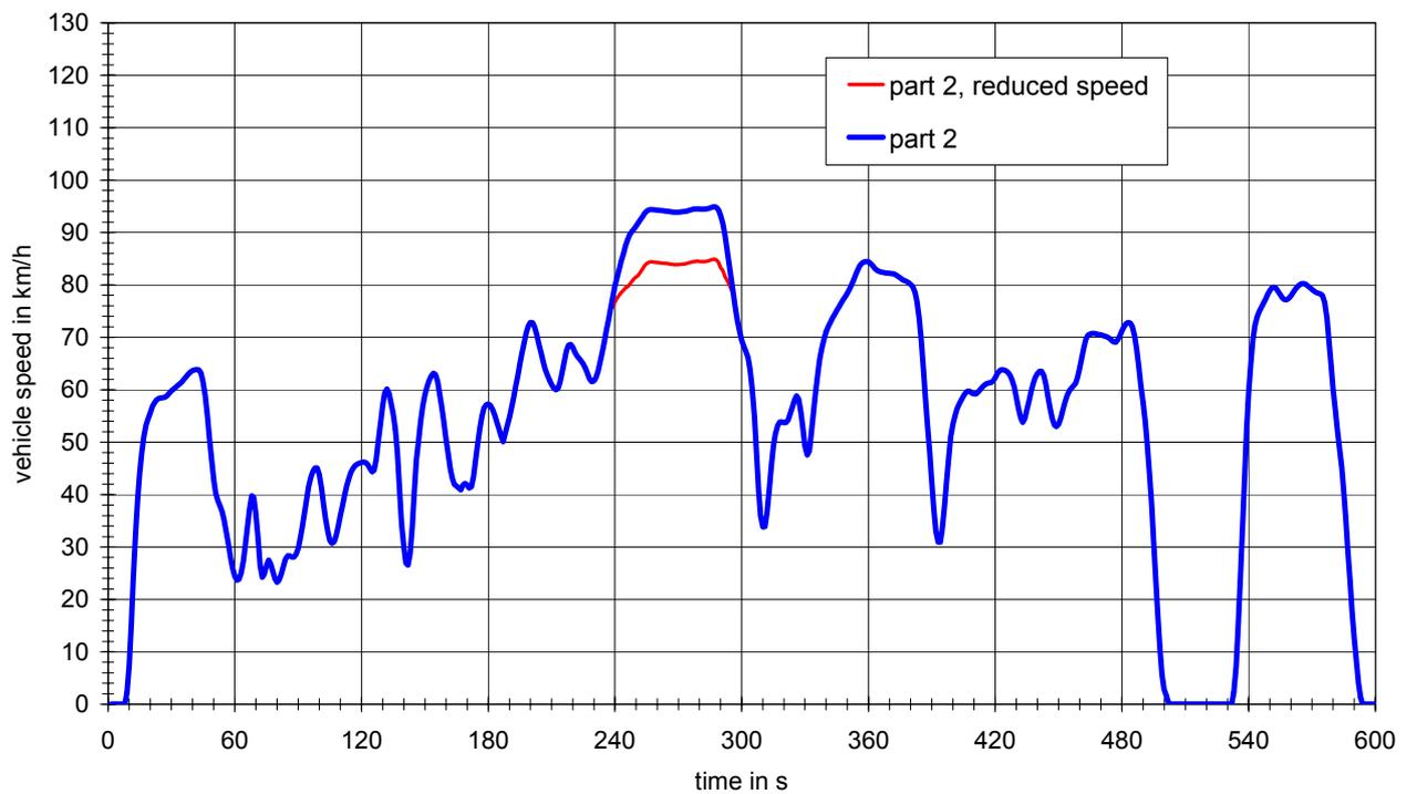
Figure A5-2: Cycle part 2 for vehicle classes 2 and 3
