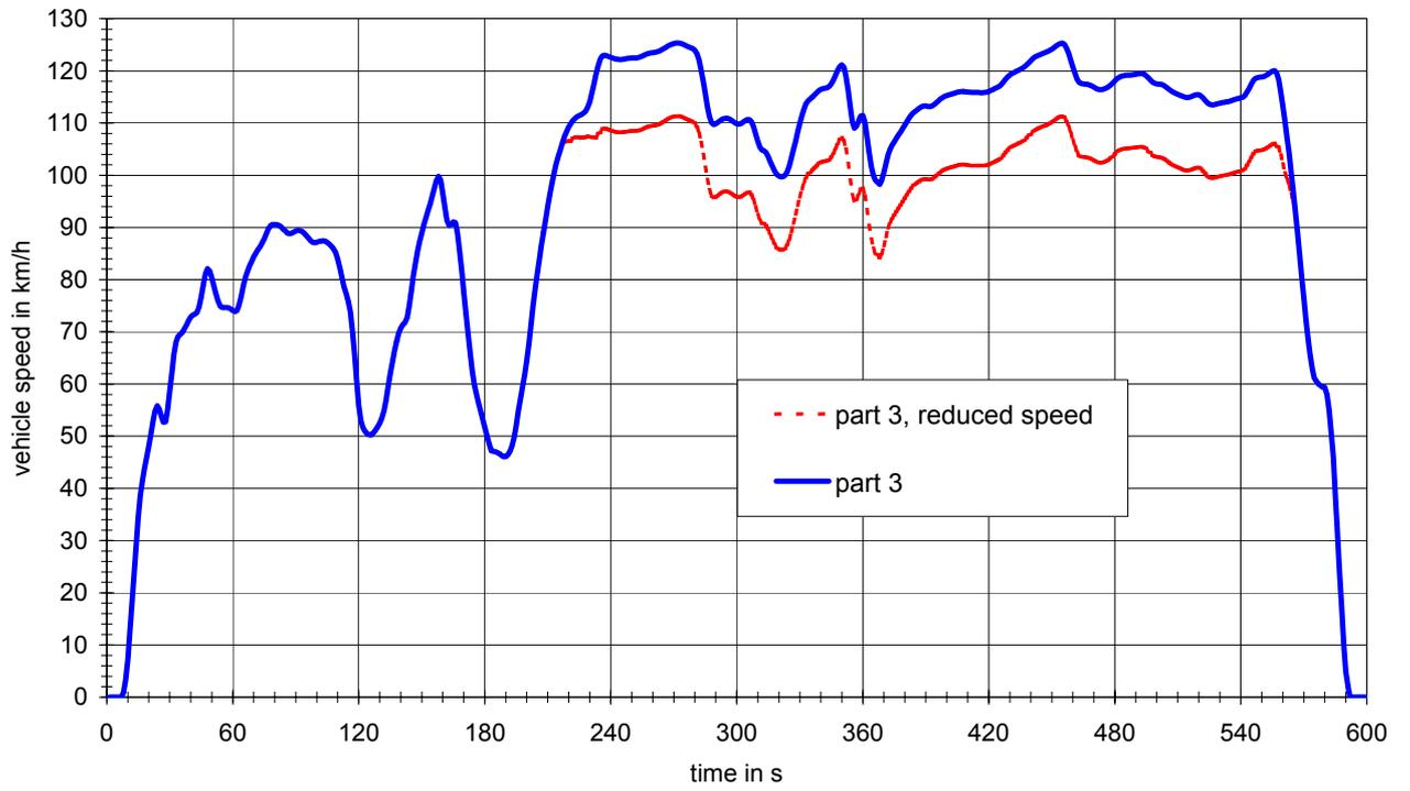
Figure A5-3: Cycle part 3 for vehicle class 3
