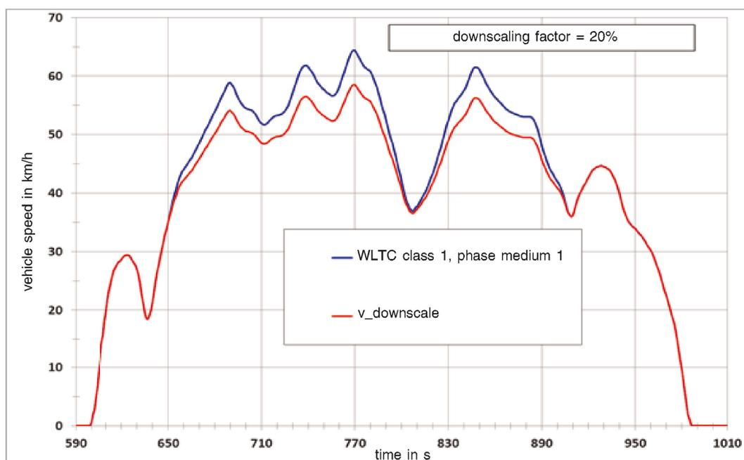
For the Class 1 cycle, the downscaling period is the time period between second 651 and second 906. Within this time period, the acceleration for the original cycle shall be calculated using the following equation:
