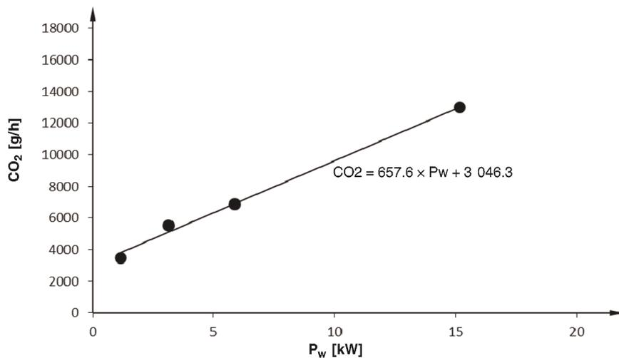
The actual wheel power shall be calculated from the measured CO<sub>2</sub> mass flow according to:
