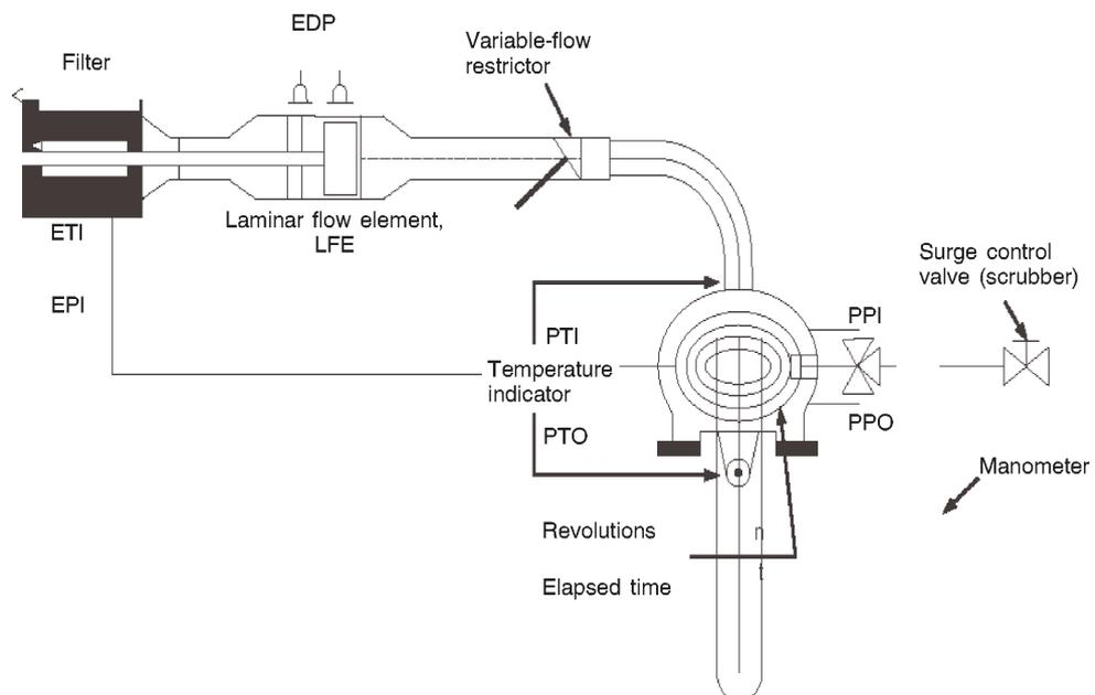
3.4.2.5. After the system has been connected as shown in Figure A5/6., the variable restrictor shall be set in the wide-open position and the CVS pump shall run for 20 minutes before starting the calibration.
