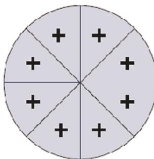
These measurements shall be made with no vehicle or other obstruction in front of the fan. The device used to measure the linear velocity of the air shall be located between 0 and 20 cm from the air outlet.
