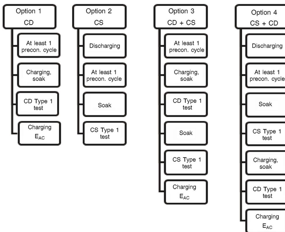
3.2.3. The driver-selectable mode shall be set as described in the following test sequences (Option 1 to Option 4).
