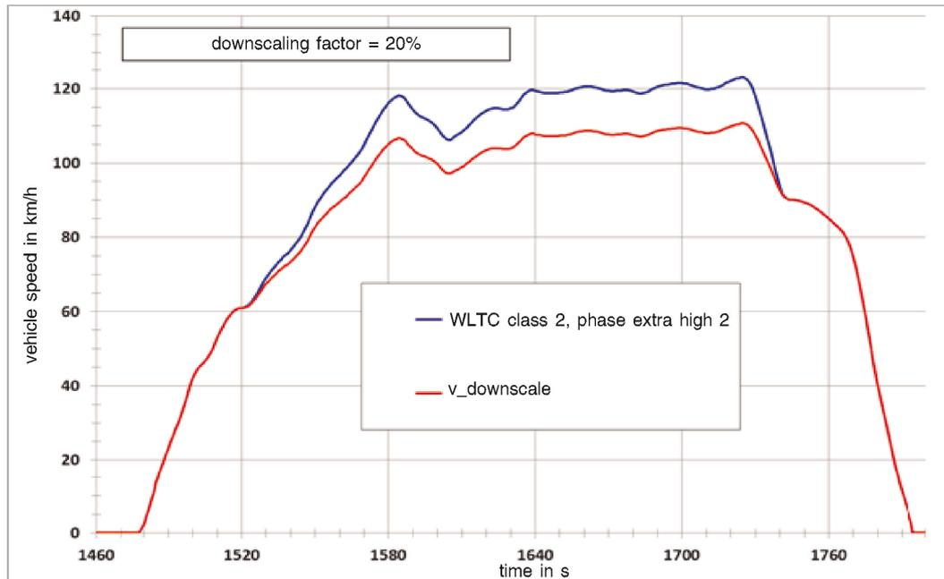
For the Class 2 cycle, the downscaling period is the time period between second 1520 and second 1742. Within this time period, the acceleration for the original cycle shall be calculated using the following equation:
