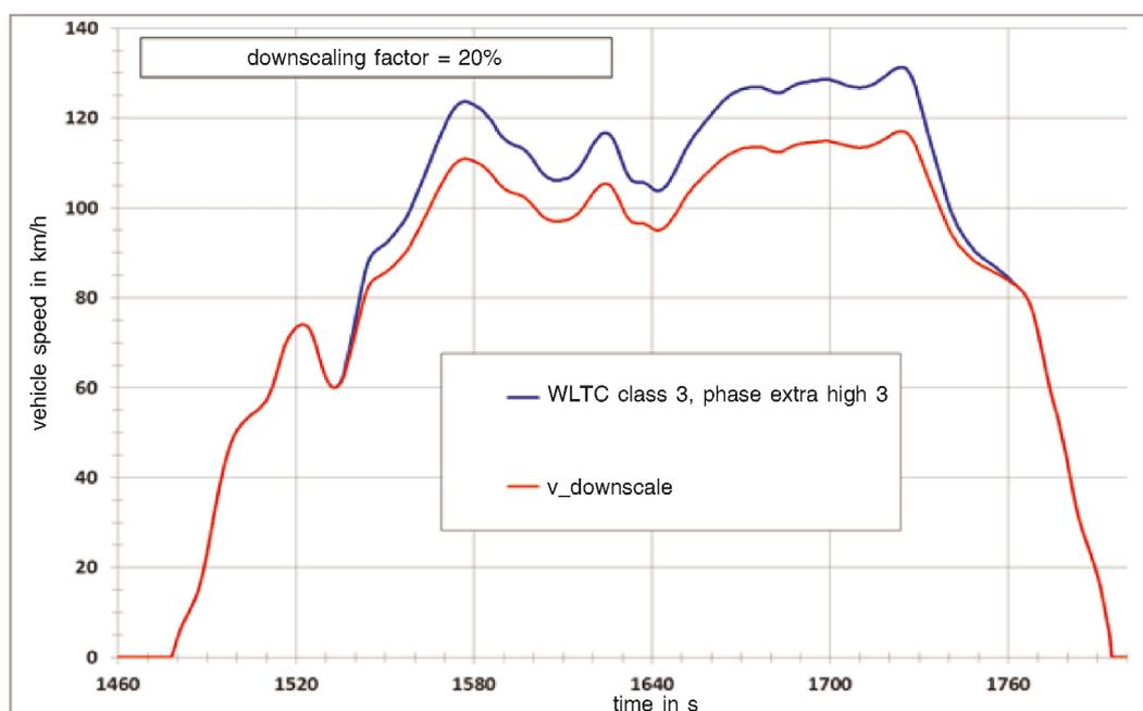
For the Class 3 cycle, the downscaling period is the time period between second 1533 and second 1762. Within this time period, the acceleration for the original cycle shall be calculated using the following equation:
