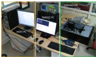
Laboratory level prototype of Real-time Simulator for EV / HEV systems
