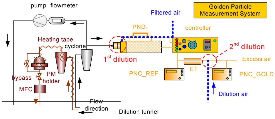
Transporting transfer and sampling components along with the measurement system avoided possible variances in the performance of the GPMS at test laboratories due to differences in installation. This left the sample probe and transfer distance between probe and PND<sub>1</sub> as the only real differences between labs' installations.
