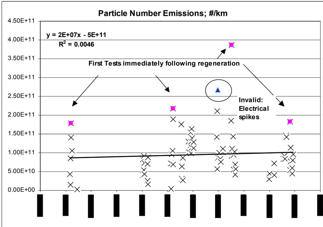
Figure 34: Electrical Spikes Increase Apparent Emissions From Au-DV#1
