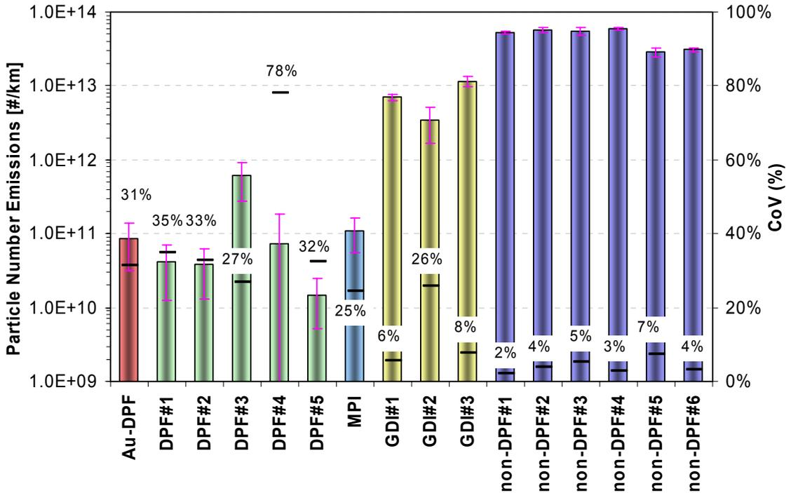
**Figure 30: Porous Wall-flow DPF Shows non-DPF-like Particle Emissions Profile**
