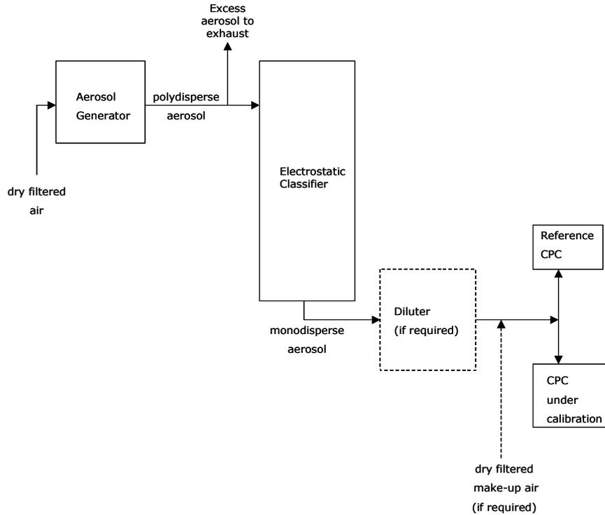
The linearity of response in terms of the  $R^2$  coefficient must be greater than 0.98, else the CPC under calibration (PNC\_GOLD) does not respond linearly over the measured concentration range. The gradient of the calibration plot must be within the range from 0.95 to 1.05 (unity signifies complete agreement between the two CPCs).
