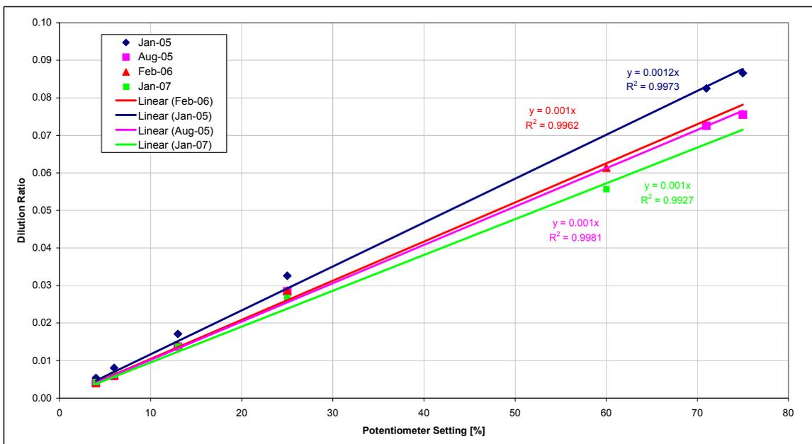
The measured dilution ratios were just outside +/- 10% of the nominal dilution ratios (as specified in the UN-GRPE PMP Phase 3 Inter-laboratory Correlation Exercise: Framework and Laboratory Guide [7]) but this is to be expected due to the difference in calibration methods between Matter Engineering (particles) and AEA (gas).
