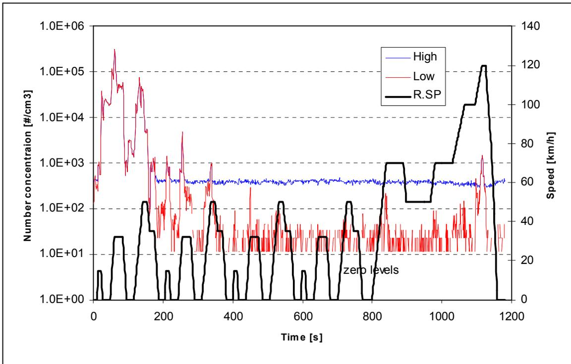
Figure 118: Effects of High and Low Particle Backgrounds On Drive Cycle Emissions
