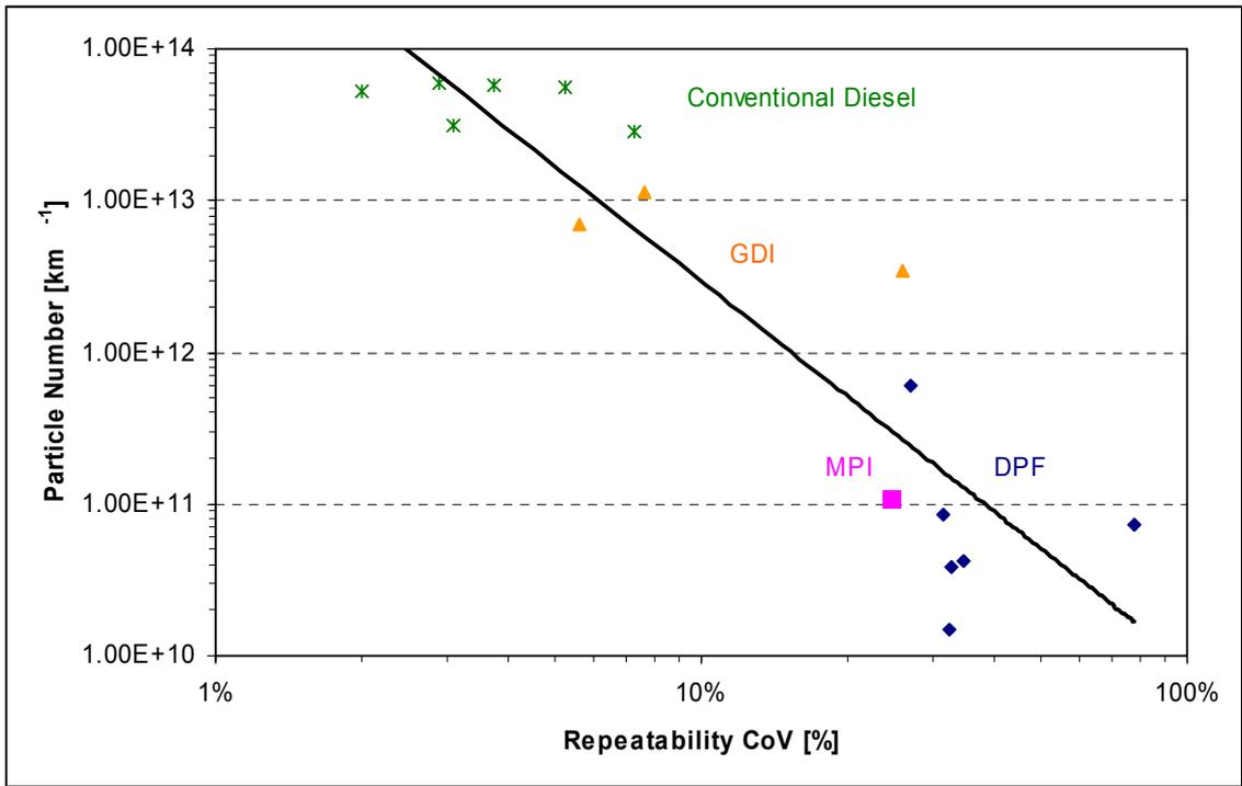
Figure 32: Particle Number Emissions Normalised to Golden Vehicle
