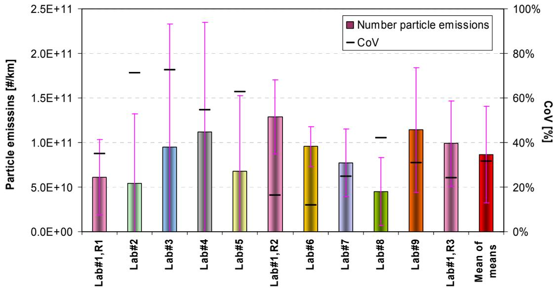
The main difference between the tests in these laboratories was the intermediate preconditioning – Lab#2 merely used 3 x EUDC between tests, rest labs used 120kph plus 3 x EUDC. In all cases, tests following a 120kph preconditioning plus 3 x EUDC generated higher emissions than those following tests with just 3 x EUDC preconditioning.
