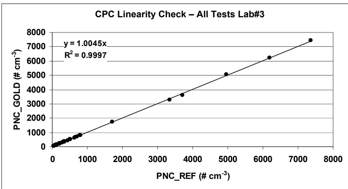
Figure 63: Daily Linearity Checks – Comparisons of PNC\_REF and PNC\_GOLD
