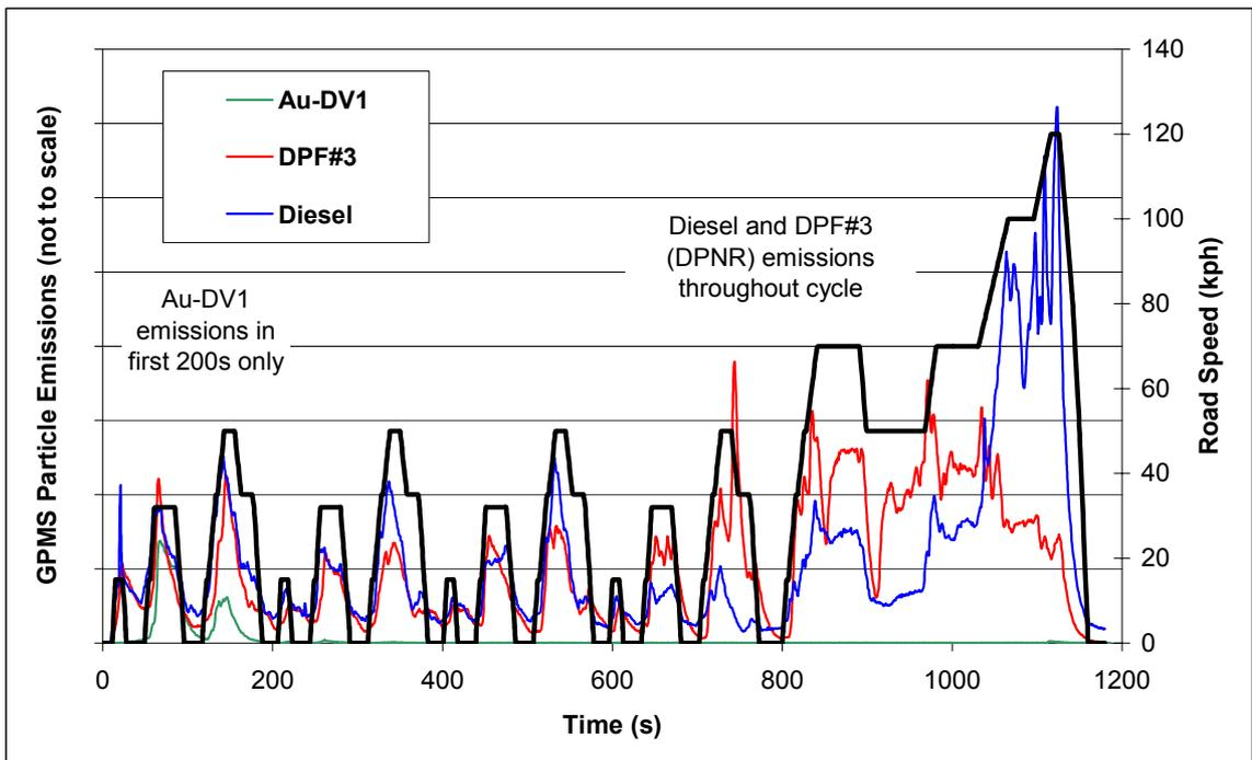
Figure 31: Particle Number Repeatability Improves with Emissions Magnitude
