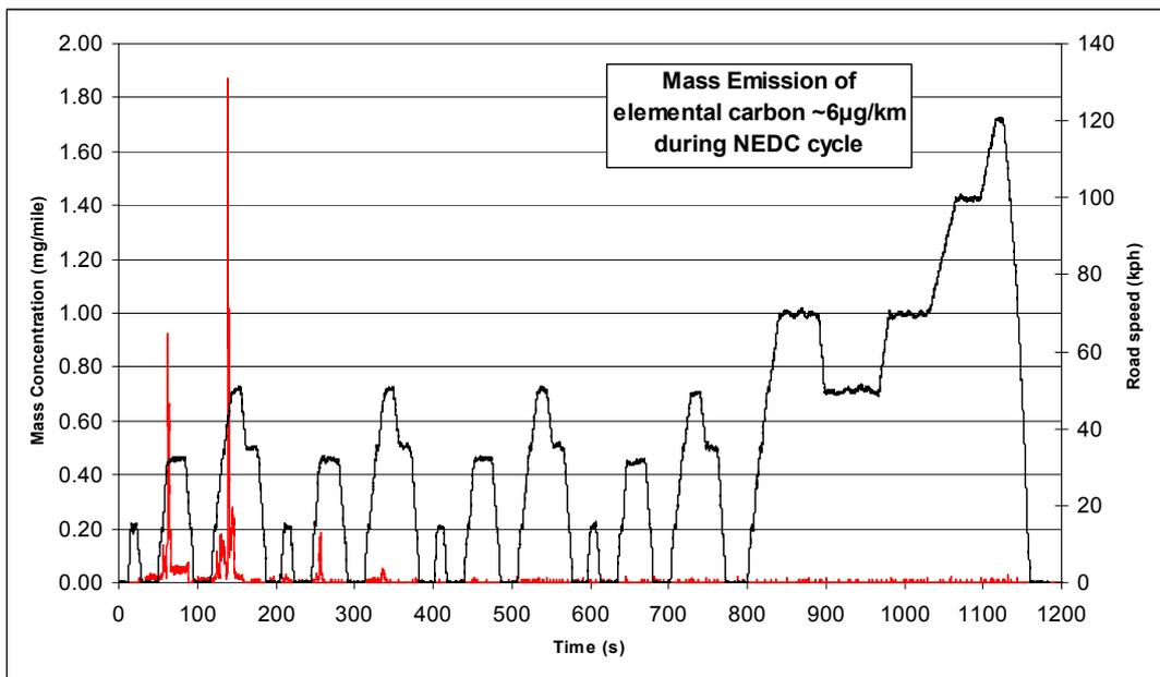
Data from the ILCE\_LD indicate that the presence of carbon is required for mass and number to correlate, and that no agreement should be expected from particulate matter
