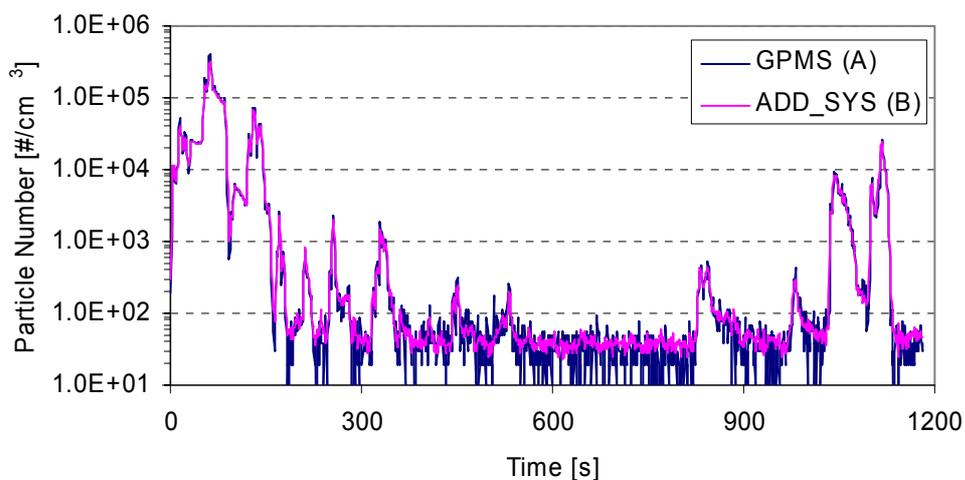
As an example for the above mentioned methods Figure 8 shows the comparison between the Golden system (method A) and the EJ+TD system in Lab#5 (method B). The scatterplot (and the regression analysis) of the two systems can be seen in Figure 9.
