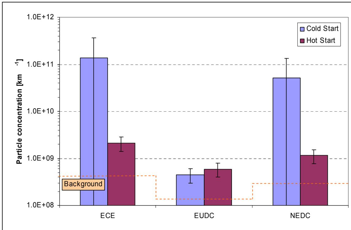
However, it is hypothesised that with the Golden Vehicle and its own particular DPF, the preconditioning process loads the interstitial voids of the DPF with carbon particles during high exhaust flows and increased engine-out carbon levels. These particles settle
