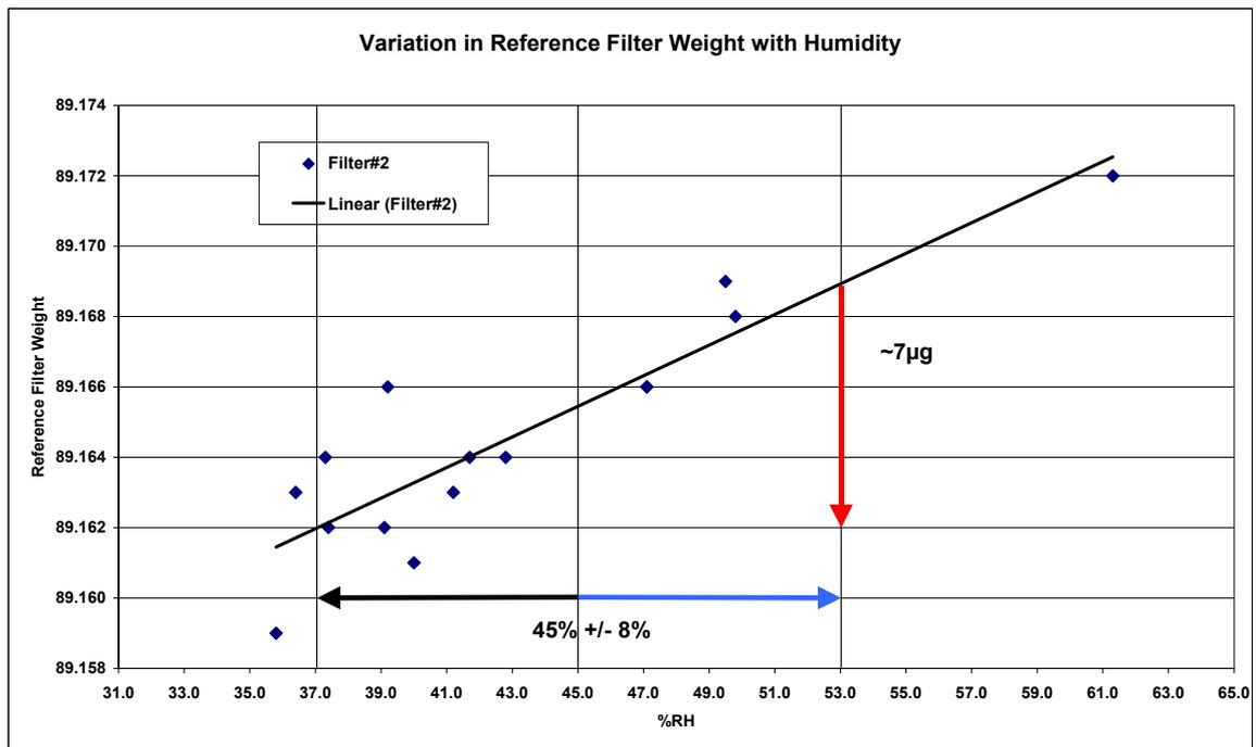
Figure 21 shows a similar trend of increasing reference filter#1 masses with increased humidity. However, with filter#1 the mass gain was less: ~4μg for the 16% increase in humidity. From Golden Vehicle tests, these variations in humidity ~7μg for reference
