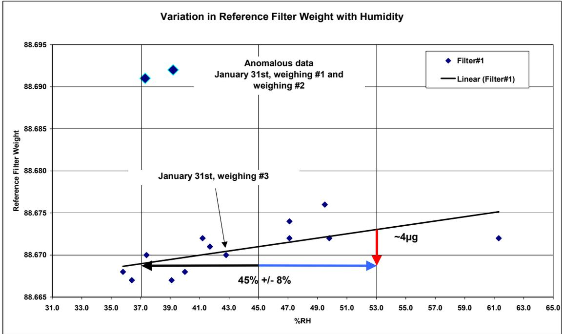
The first two weighings of filter#1 on January 31<sup>st</sup> were anomalously high, both in the light of a subsequent weighing and the fact that filter#2, which was weighed at the same time, did not show the same elevated masses.
