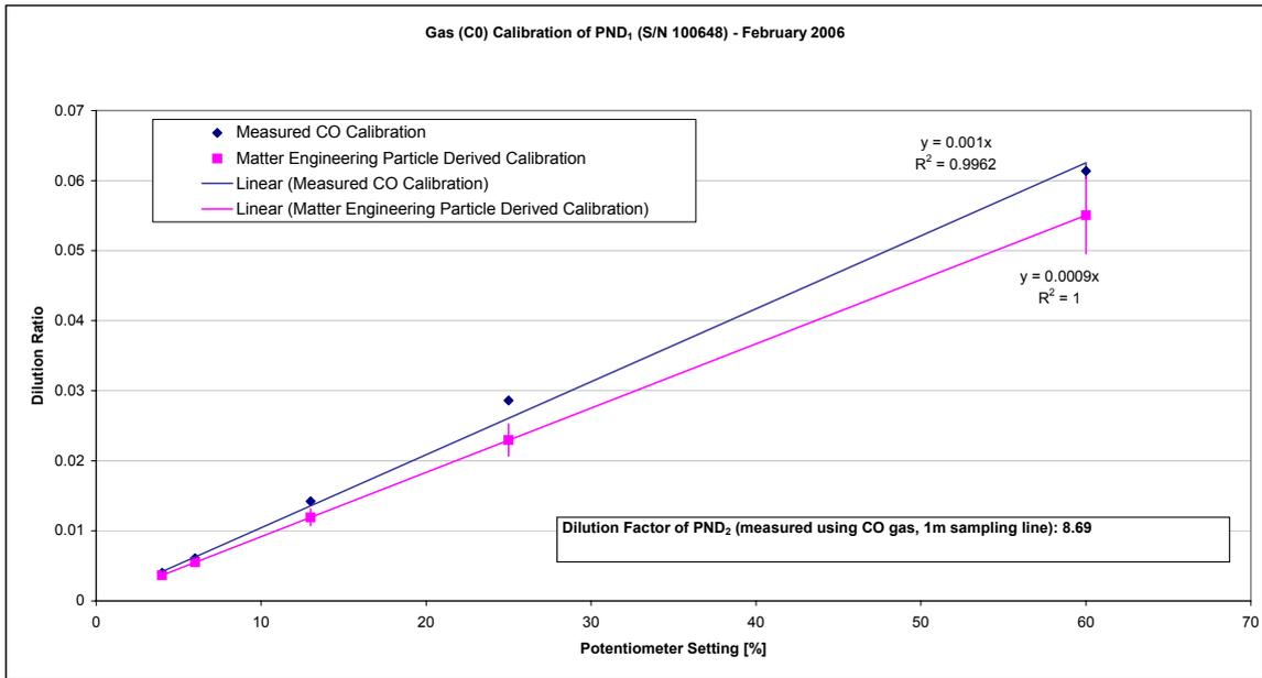
The pink line represents the particle-derived calibration from Matter Engineering and the blue line is the gas calibration performed by AEA. The accuracy of both measurements are shown using error bars. The calibration equations used to produce the Matter Engineering data (pink line) are as follows (taken from their particle calibration reports):
