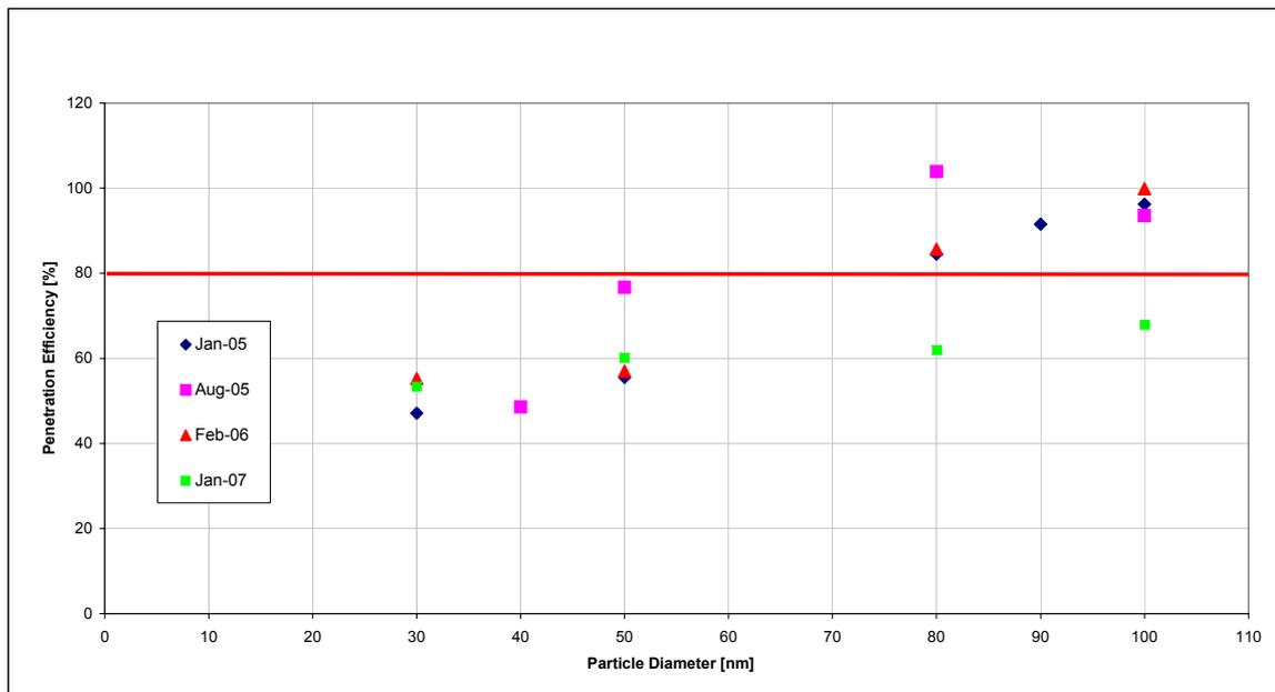
The PE data has been re-analysed using the dilution factors measured by AEA during each gas calibration. This ensures that the particle concentrations are compared with the expected concentration using a dilution factor that does not include any particle losses. This method assumes 100% of the particles entering the diluter are diluted by a known amount (using the gas dilution factor) and no particle losses occur.
