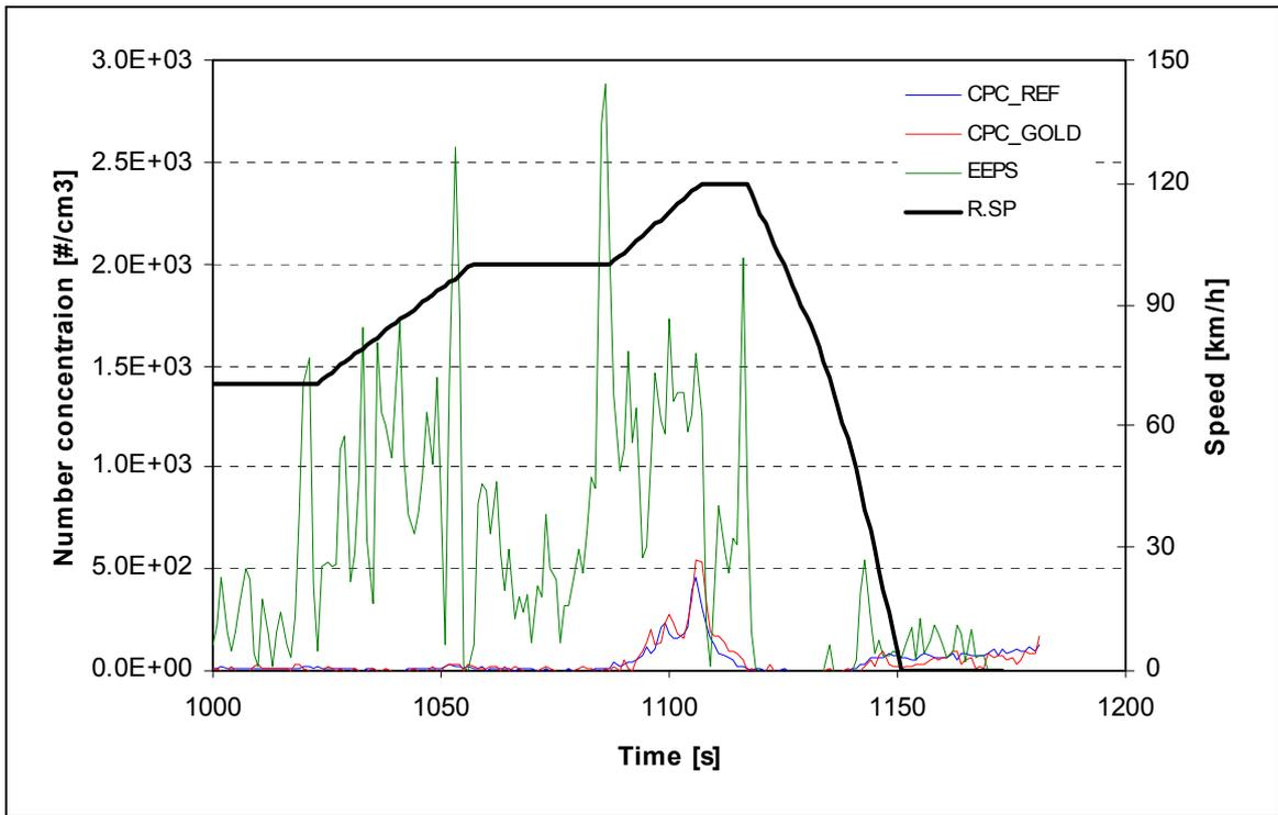
Similarly, during a 120kph steady state (Figure 66) emissions levels from PNC\_REF and PNC\_GOLD are highly similar: no semi-volatile particles penetrate the initial hot dilution stage at this operating condition.
