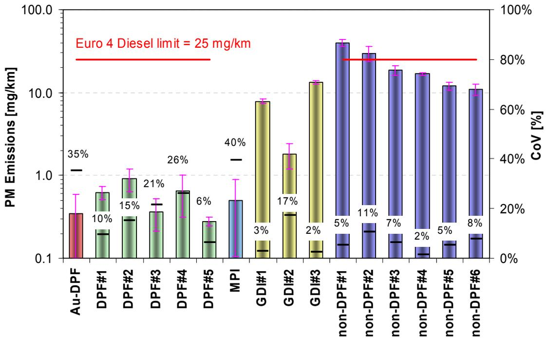
The highest emitting Euro 4 Diesel vehicle produces ~120x the PM emissions levels of the Golden Vehicle, and the lowest emitting ~30x (Figure 14).
