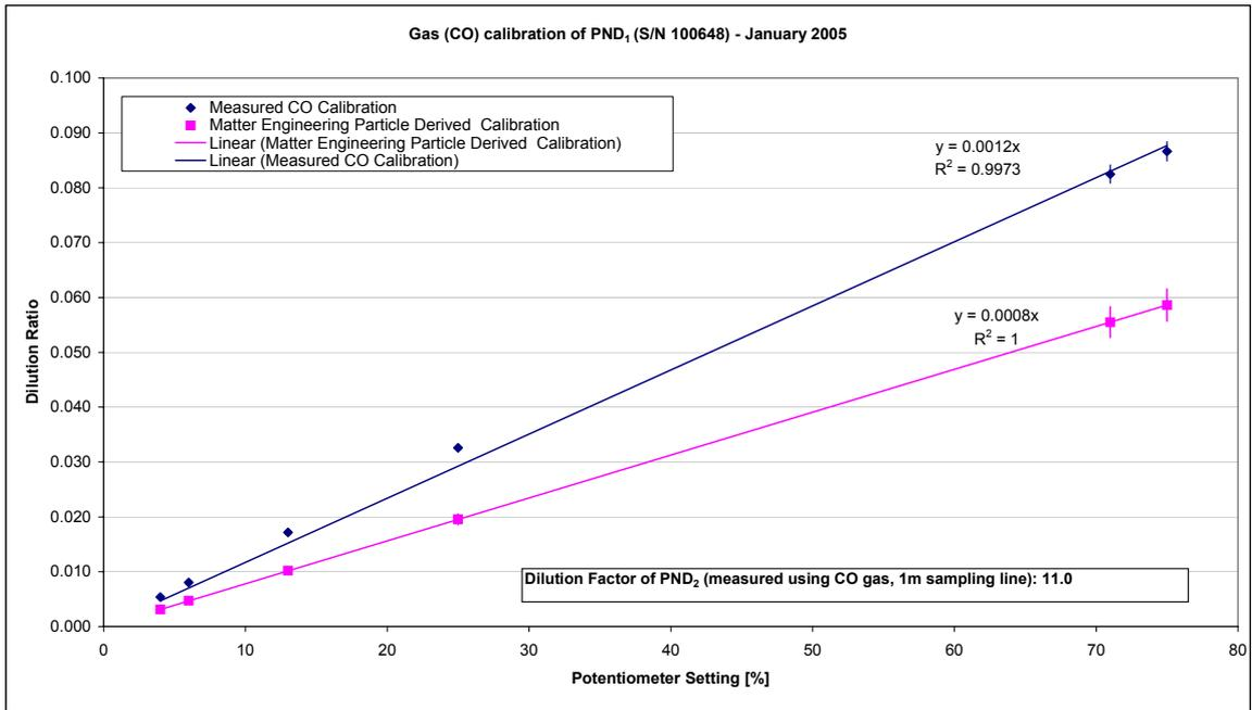
**Figure 37: Calibration of PND<sub>1</sub> using CO gas – August 2005**
