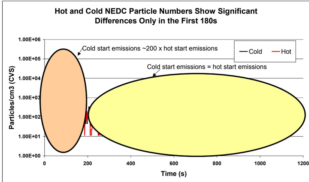
**Figure 89: Comparative Cold and Hot NEDC, ECE & EUDC Particle Number Emissions**
