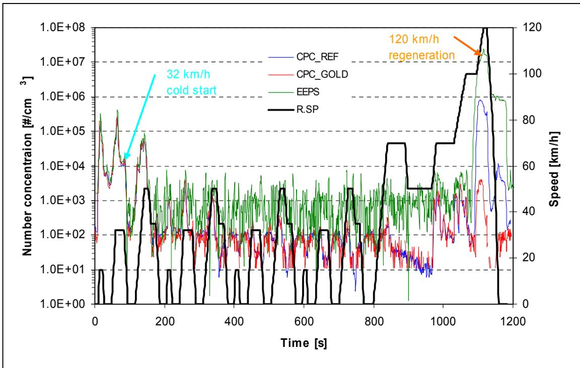
However, when a regeneration is observed during the EUDC phase of an NEDC (Figure 69), elevated particle levels are seen in >6nm, >22nm EEPS data and also after PND<sub>1</sub> (Figure 70). In this case the very low volatility particles emitted in response to the high
