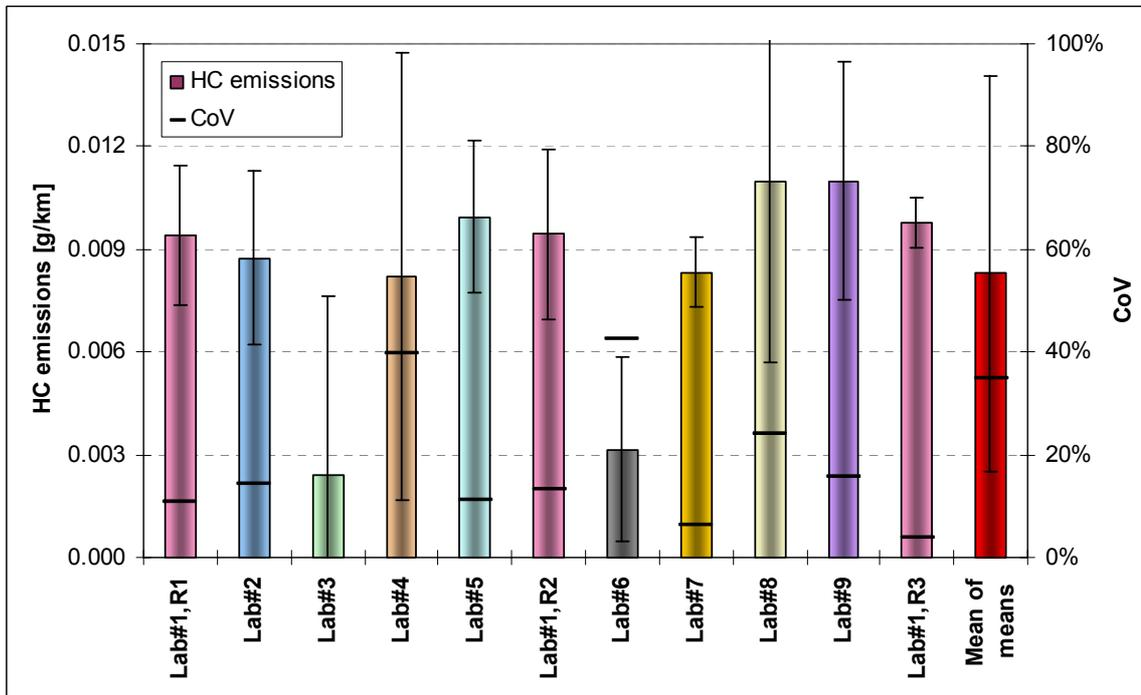
As observed for CO, hydrocarbon emissions (Figure 101) from the Golden Vehicle were also low and varied from lab to lab in the range 2 to ~10mg/km.
