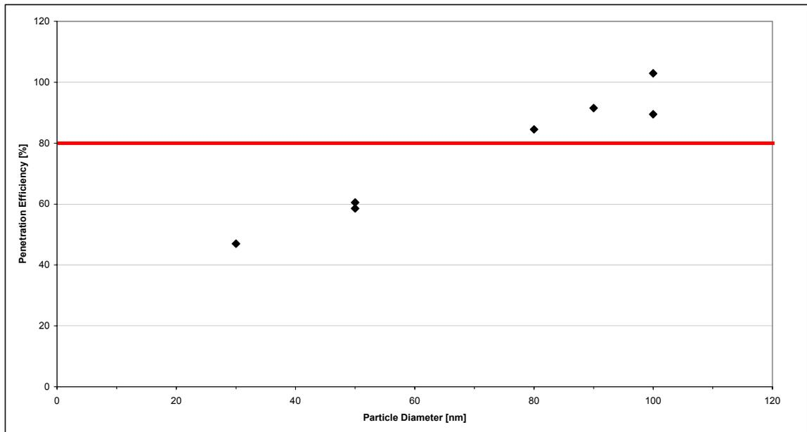
**Figure 42: Penetration of monodisperse solid sodium chloride particles – August 2005**
