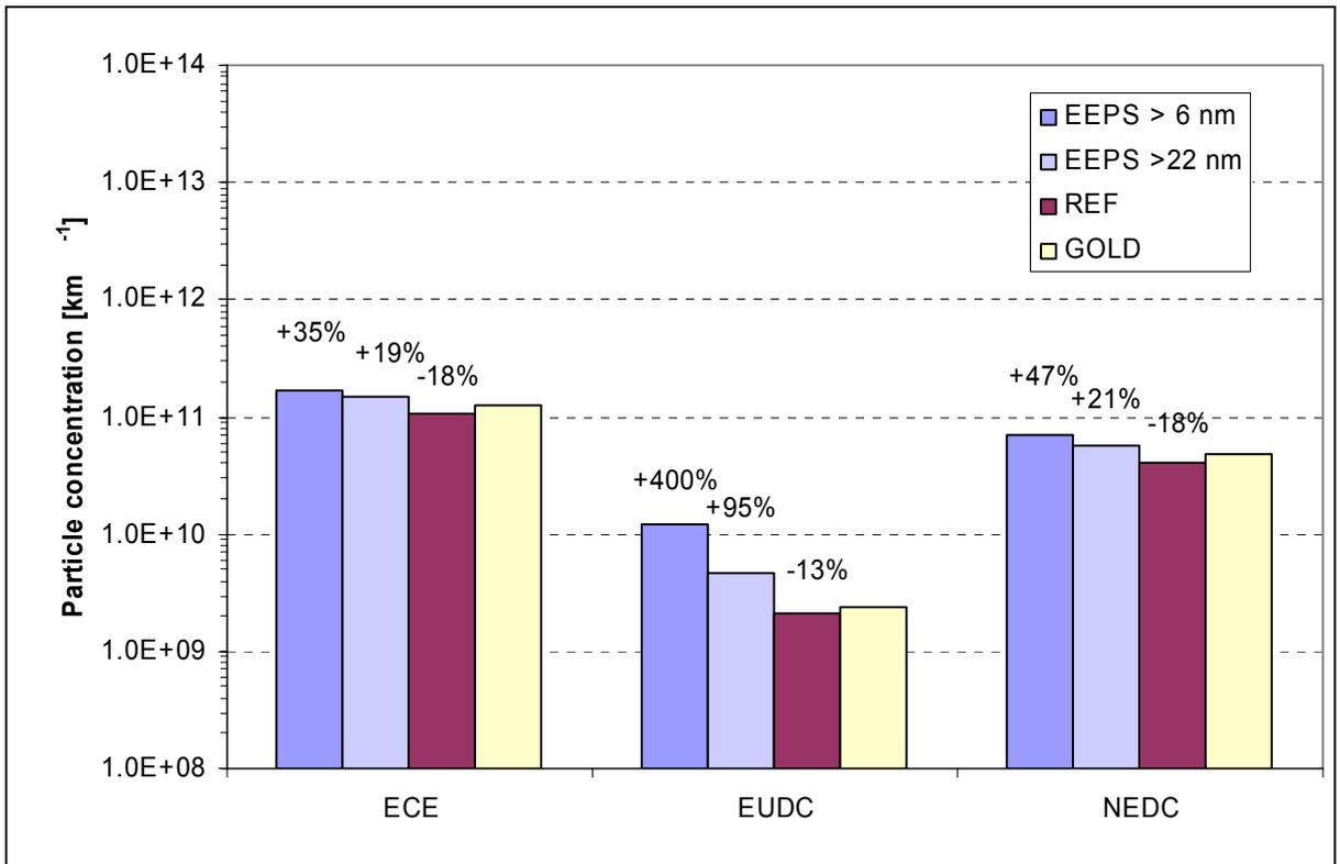
Figure 69: Particle Number Emissions, NEDC with EUDC Regeneration
