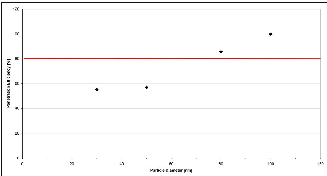
**Figure 44: Penetration of monodisperse solid sodium chloride particles – January 2007**
