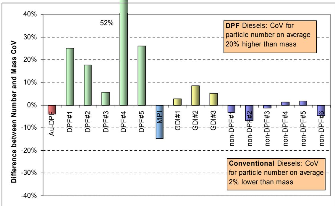
What is clear from these results is that data from a stable particle source (conventional diesels) show that the particle number method is both substantially more sensitive and more repeatable than the mass method employed in PMP.
