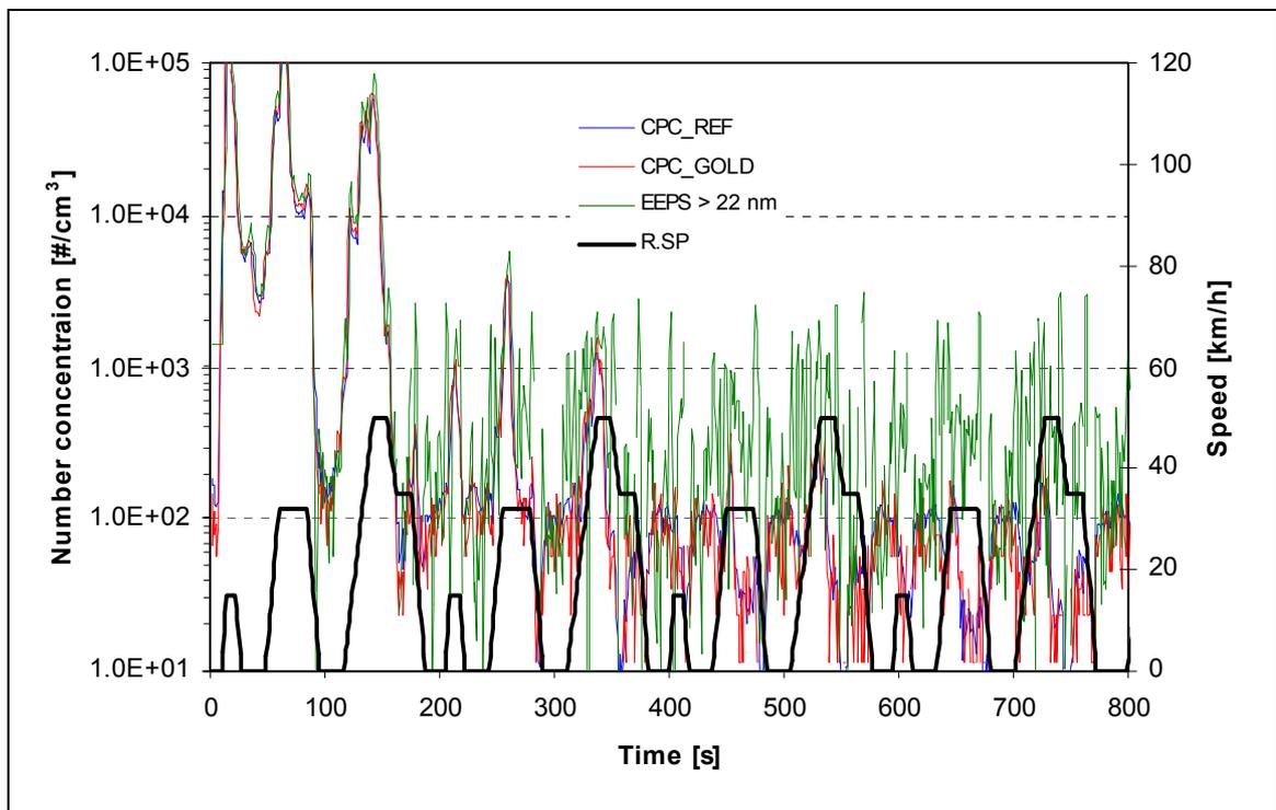
Data from the EUDC shows that volatile particles are also emitted at the end of the NEDC cycle (Figure 65) but after PND<sub>1</sub>, only solid particles remain.
