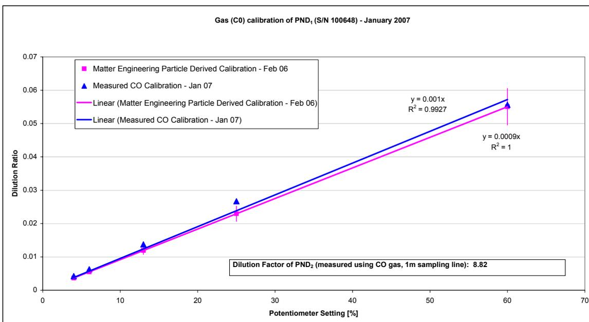
*Note:* PND1 was repaired by Matter Engineering in December 2006. The dilution block and disc were replaced due to excessive wear. Matter Engineering did not perform a particle calibration after this repair work and hence the dilution factor has not changed between the February 2006 and January 2007 calibrations.
