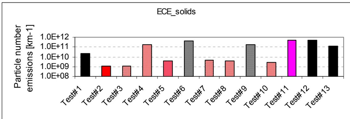
Differences in emissions during ECE cycles can be attributed to types of preconditioning, effects of soak period, hot and cold starts, DPF filtration efficiencies and regeneration influences (Table 17:).
