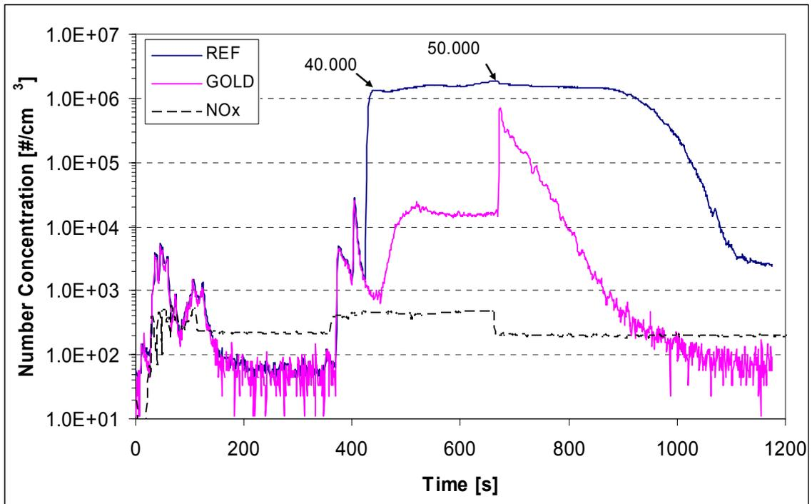
If regulatory procedures for particle numbers are to address regenerations, both hot dilution and an evaporation tube will be required. If an ET is required, the use of a secondary diluter (PND<sub>2</sub>) at >10:1 dilution will also be essential – to reduce the temperature of the aerosol sample from ~300°C to <35°C prior to entering the PNC whilst avoiding thermophoretic losses.
