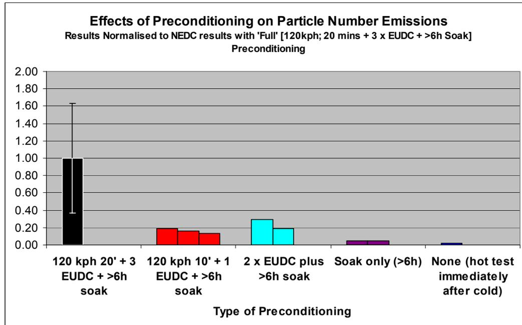
Experiments investigating preconditioning effects on particulate mass emissions showed no obvious effects (Figure 22, Section 4.3.6). This was not the case with particle number measurements: there were clear effects. In general, particle numbers from NEDC cycles decreased as the severity (in terms of speed and load) of the preconditioning decreased (Figure 87).
