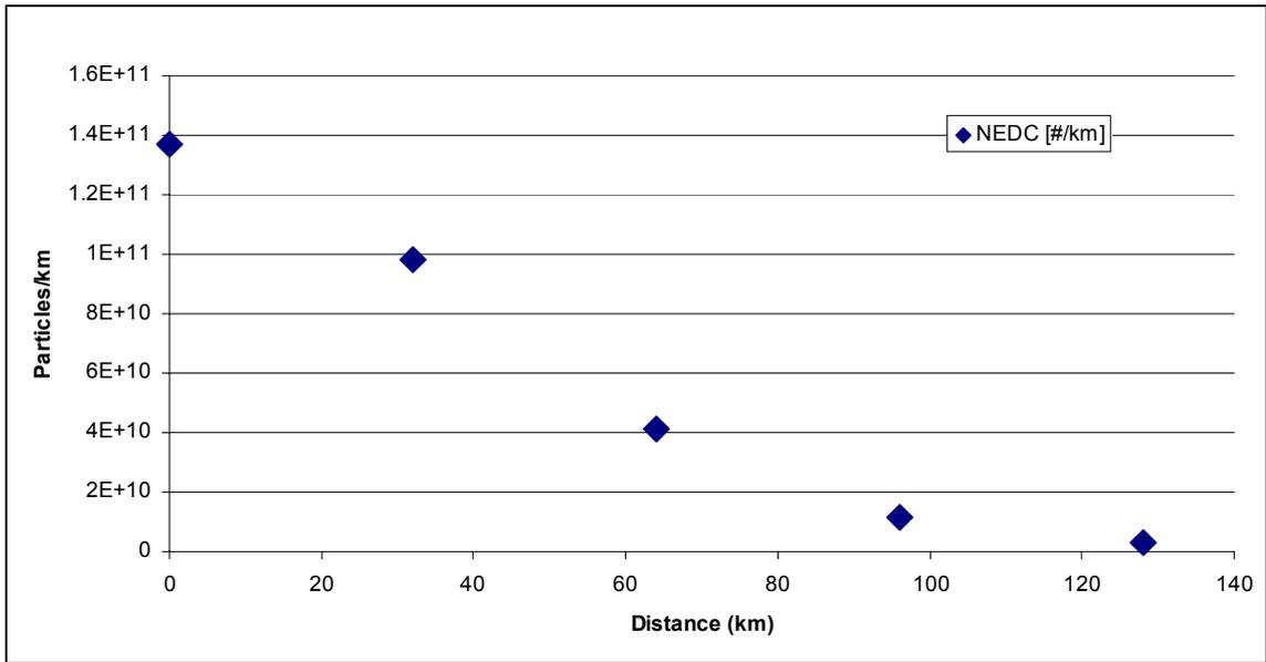
The exception, DPF#4, was the LDV: this experienced a scheduled regeneration directly before the first NEDC test and showed a continuous reduction in particle numbers as mileage increased (Figure 28) and the DPF filled. Note that the final test shown in this chart is omitted from the ILCE\_LD dataset as a particulate mass outlier. The high (78%) variability quoted for DPF#4 was calculated from the first 4 tests only.
