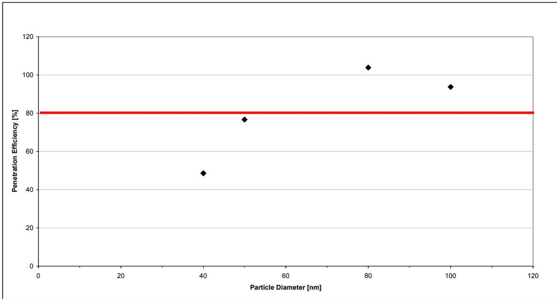
**Figure 43: Penetration of monodisperse solid sodium chloride particles – February 2006**
