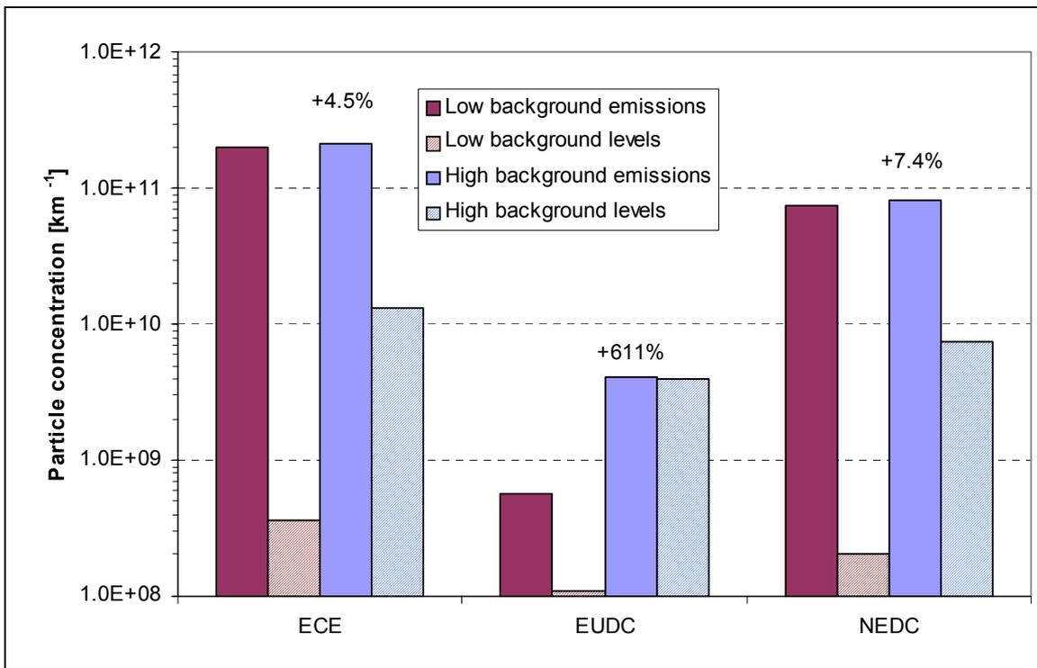
There is a large discrepancy between the possible contribution of a filter background to a sample measurement, and the possible contribution of a number background: in the Lab#1,R3 tests >100% and ~0.2% respectively. The high mass contribution to the filter measurement must come from the dilution air or from volatiles emitted from the dilution tunnel walls since the number method shows minimal levels of solid particles to be
