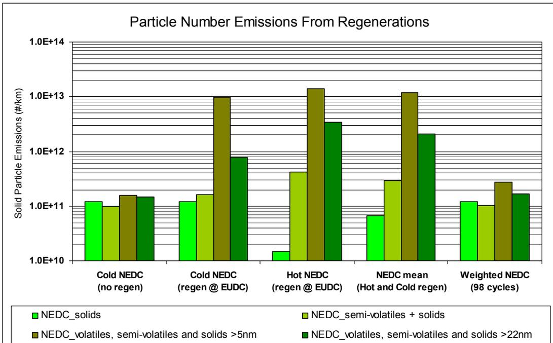
Interestingly, from this series of regenerations, it was calculated that an NEDC cycle containing a complete regeneration would produce solid particle emissions similar to a non-regenerating test and when this contribution is divided across 98 tests, there is no effect on the weighted emissions rate.
