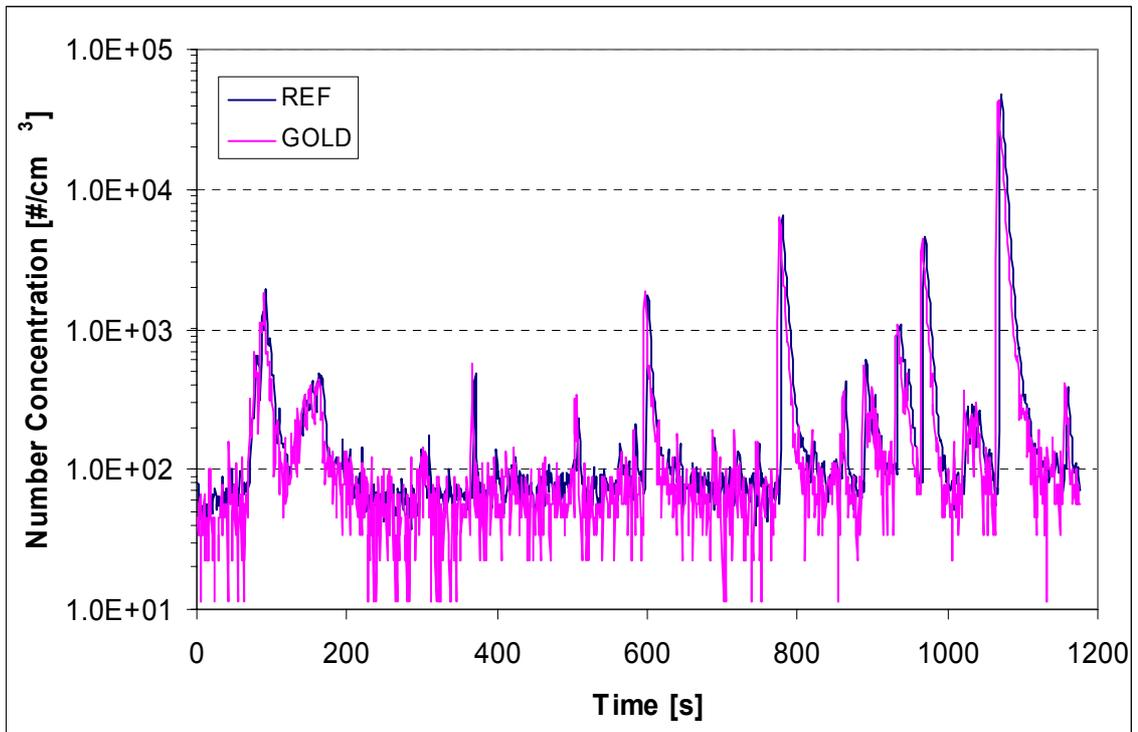
However, when an active regeneration is observed during a 120kph steady state (Figure 67), many volatile particles are observed and the ET is required. Of the particles that
