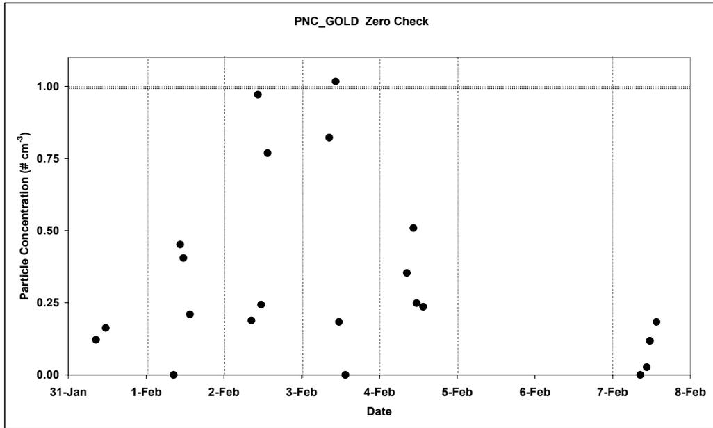
The reference CPC did not exceed the 1cm<sup>-3</sup> permitted response at any time during the testing period.
