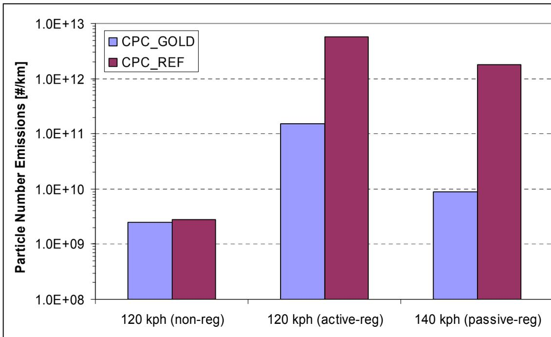
During the passive regeneration soot oxidation may be more efficient than from the active regeneration due to a surplus of oxygen, and exhaust temperatures will be lower:
